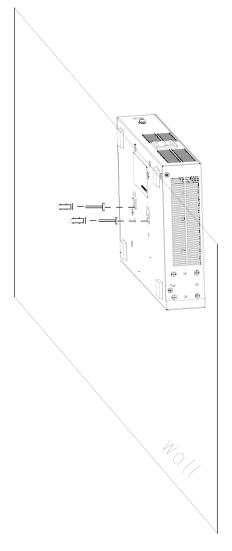
WARNING! The Switch should be wall-mounted horizontally, and make sure the front panel is facing down. The Switch's side panels with ventilation slots should not be facing up or down as this position is less safe.
